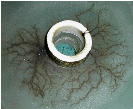
picture 16: the sliding discharge on a board out of polycarbonate leading to the destruction of the insulator
