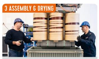
We use high-grade core material with step-lap design to reduce no-load losses and noise.
