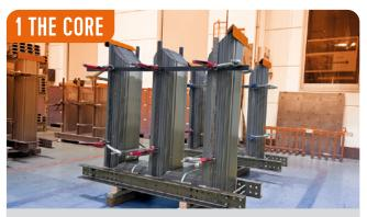
Active parts are assembled short-circuit proof and undergo vacuum drying for maximum impregnation.
