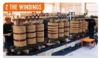
LV winding uses foil technology for high short-circuit resistance. HV winding uses enameled round wire.
